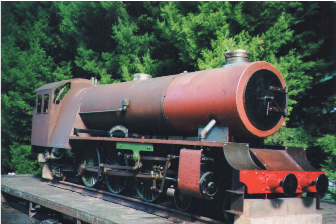
Thurston used some of parts from the above locomotive to build a 4-4-2 - also for his line on Hayling Island. The incomplete 4-6-2 passed into the ownership of Ted Martin, who as we see here, constructed a rather more attractive cab (as well as a new tender, the original one having been scrapped in the intervening years). The locomotive is on a trailer having returned from being displayed at the Knowl Hill Steam Rally.
